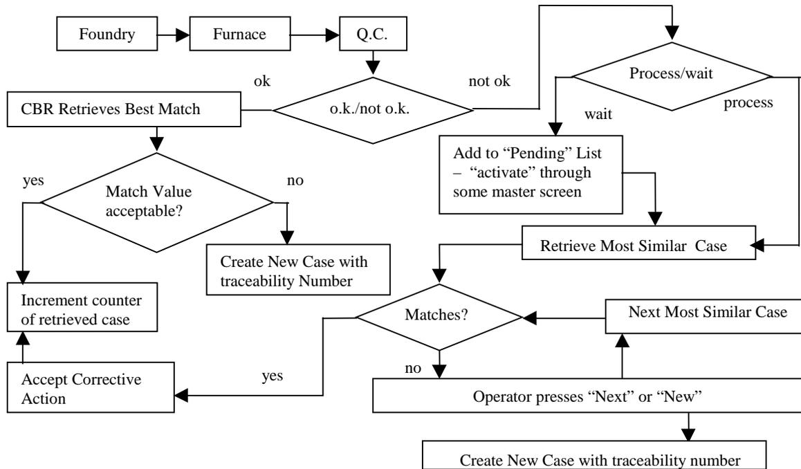
Fig. 3 Flow Diagram for the integrated System
