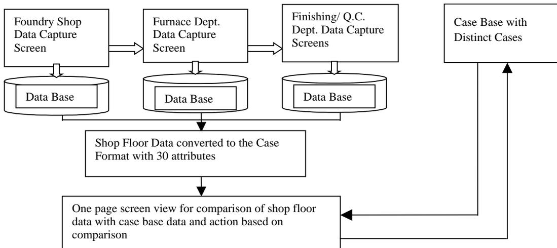
Figure 3: Flow chart for the integrated system
