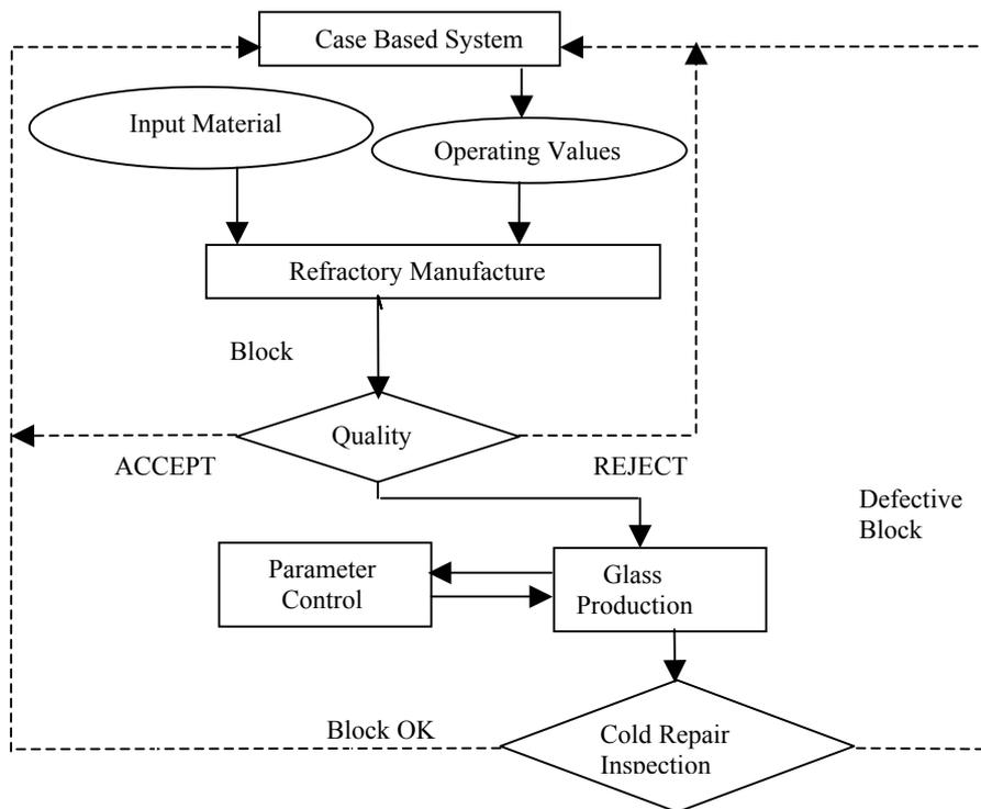
Fig. 2. Role of CBR in Refractory and Glass Manufacture
